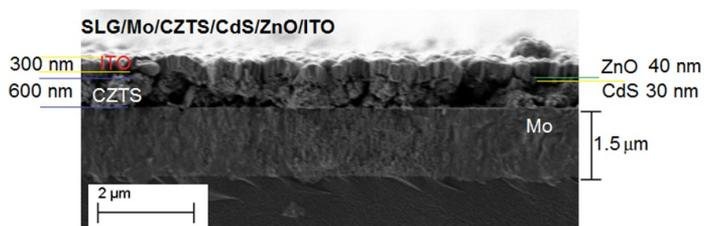
**Fig. 9.** Cross section of SLG/Mo/CZTS/CdS/ZnO/ITO solar cell device.
