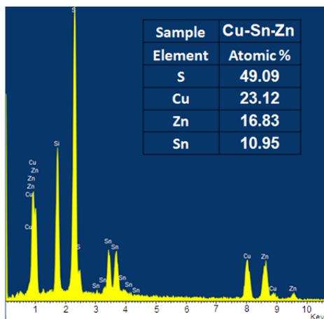
**Fig. 7.** EDS analysis for co-evaporation sequence Cu/Sn/Zn.
